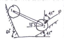
c) Just before they collide, two disk on a horizontal surface have velocities shown in fig. Knowing 06 that 90N disk 'A' rebounds to the left with a velocity of 1.8 m/s. Determine the rebound velocity of the 135 N. disk 'B' Assume the Impact is perfectly elastic.
