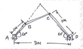
Q.5 a) In the truss shown in fig. compute the forces in each member
